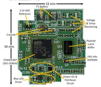
The photo in the left column shows the core of a BMR-STM32-VPX IPMC. The active components are:
